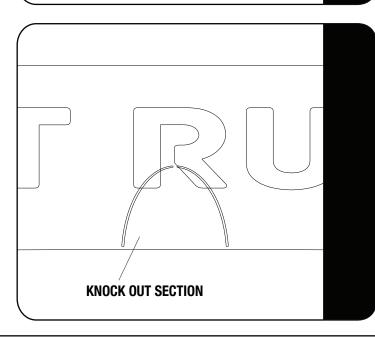
If your vehicle has a Roof Antenna which interferes with the Wind Fairing touching the roof. The knock out section can be removed.
