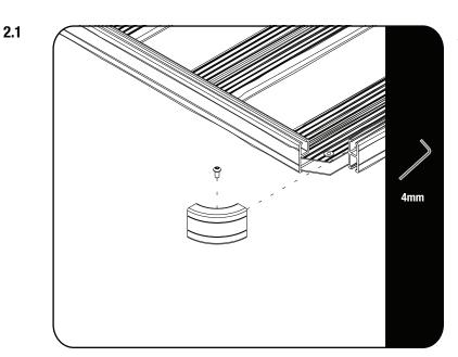
Start with removing the front right-hand Corner piece with a 4mm Allen Key.
