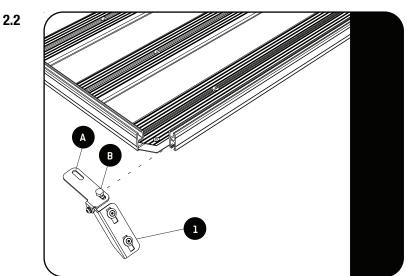
Adjustable Brackets (Item 1) into the bottom T Slot as shown. Use either Slot A or B as shown in Figure 2.2.
