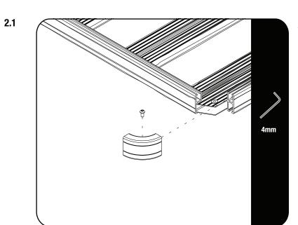
Start with removing the front right-hand Corner piece with a 4mm Allen Key.
