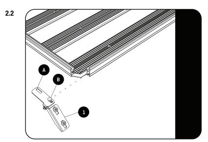
Slide 4 loosely assembled Wind Fairing Adjustable Brackets (Item 1) into the bottom T Slot as shown. Use either Slot A or B as shown in Figure 2.2.
