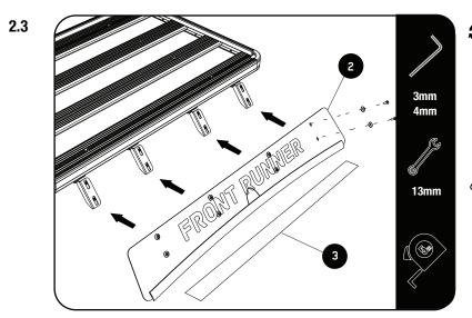
Remove the M5x16 Countersink Screws & M5 Finishing Washers from the bracket.
