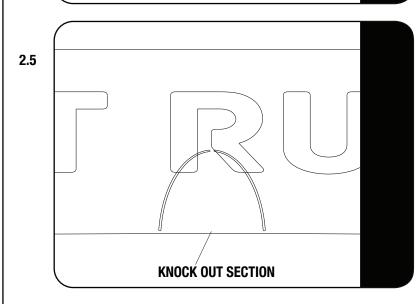
If your vehicle has a Roof Antenna which interferes with the Wind Fairing touching the roof. The knock out section can be removed.
