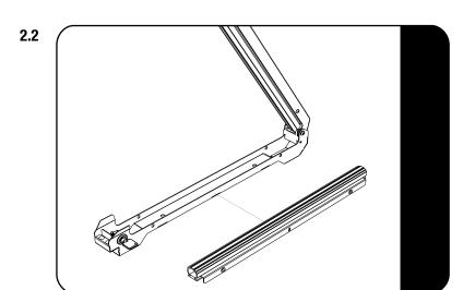
With the Carrier in the open position, remove the Rubber Extrusion and Clamping Plates as shown. Keep the Plates and Extrusion together as one unit when removing.
