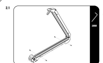
Unlock and open the Carrier (Item 1). Loosen and remove the four M5 Button Head Bolts in the base of the Carrier as shown.
