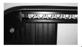
( **B** ) On the back of the Awning, slide three M6 x 16 Hex Bolts (Item 2) into the top and bottom extrusion slots as shown.
