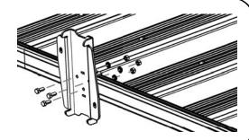
( C ) On the back of the Awning, slide three M6 x 16 Hex Bolts (item 1) into the top and bottom extrusion slots as shown.
