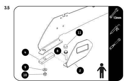
Apply a bead of sealant on the threads of the M8 x 40 Flange Bolts (Item 8) and in the cut outs in the Front and Rear Spacers (Items 4 and 5).
