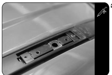
Place a bead of Sealant on the Ditch Trim before placing it back into the vehicles ditch.
