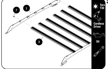
Assemble the Footrails (Item1) to the six rear slats (Item 3) (Leave the first slat unassembled for now) using M6 x 25 Thread Forming Screws (Item 7).
