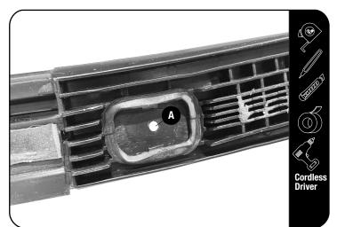
**Remove the Ditch Mold from the vehicles** roof. Remove the Stud insert from the plastic trim and place the Bottom Spacer (Item 6) into the opening and mark the center of the hole (A).
