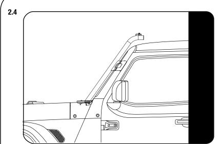
Angle the bar so that it is parallel to the door shut line.
