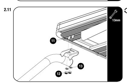
When you get to the front bars, check support bar alignment with door shut line before tightening to the rack. (The top has slots and will allow it to be adjusted).
