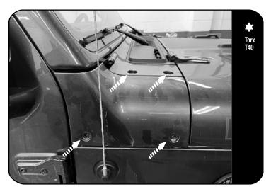
Using a T40 Torx driver, remove the 4 bolts securing the cowling cover as shown.
