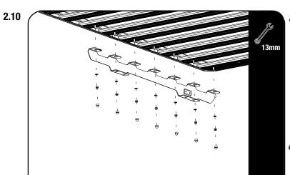
With the help of a friend place the rack onto the rails and brackets. Position all the bolts so that they drop through foot rail slots and the front mount bars. Center the rack.
