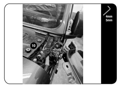
Refit the cowling cover and place the spacers (item 10) in the top two recesses as shown.
