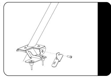
Loosely fit the inner bracket (item 5) to the bracket weld assembly (item 1) and support bar (item 1). Place the assembly over the top 2 mounting points (10) shown below in 2.3 and fit the two bolts (item 8).
