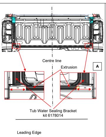
2.4) Measure and position the aluminium extrusion's (668AM002) centre between each of the rear tailgate sealing brackets (A).
