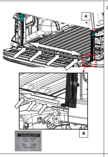
2.2) With the tailgate open, clean the entire length of the rear vertical face of the rear tub floor, between the lower ends of the tailgate sealing brackets as assembled to the vehicle shown at (B) with the alcohol wipe (6602018).
