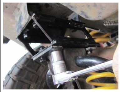
Raise the sway bar to meet the brackets and install the remaining M8 fasteners as shown.
