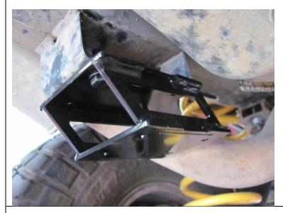
Remove the front sway bar and install the brackets with the M8 bolts, washers and flange nuts as shown.
