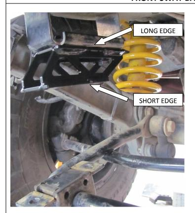
Remove the front sway bar and install the brackets with the M10 bolts, washers and flange nuts as shown.
