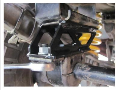
Raise the sway bar to meet the brackets and install the remaining M10 fasteners as shown.
