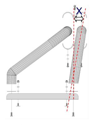
WARNING: fit the N and O front bends as shown in the drawing
