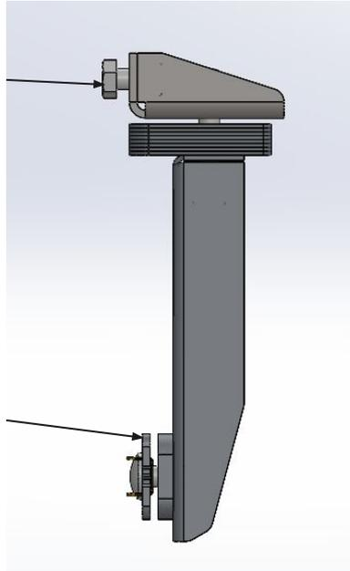
With the nut plate assembly fitted in the rail line the cup squares up with the holes on the NP300 channel bracket.
