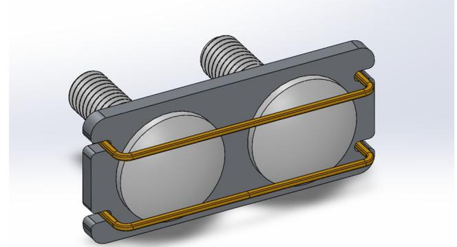
Assemble the nut plate, cup square and elastic band as shown in the image above. Slide this assembly into the rail in the load bin
