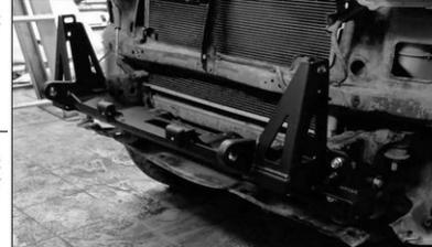
19. Mount winch bracket (2). Use OE bolts and supplied bolts M10x30 (17), bolts M10x25 (16), washers M10x20 (29), washers M10x30 (30) and nuts M10 (26) from the fitting kit bag.
