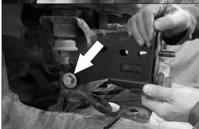
16. Mount support bracket (3) and fix it with bolt M12x30x1,25 (18) with washer M12x37 (31).
