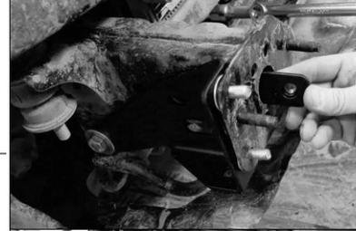
18. Place insert nut 2xM12 (9) inside of the chassis. Screw on bolts M12x30 (19) with washers M12x37 (31).
