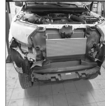
10. Remove the bumper by pulling the bumper towards you holding the sides.
