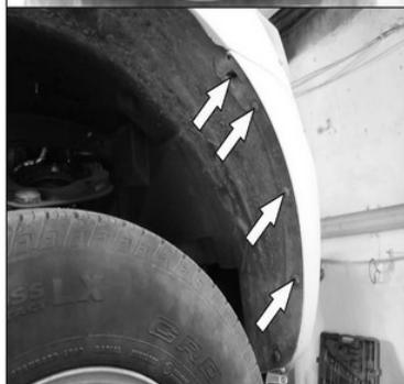
4. Remove 3 screws from inside of the fenders on each side of the vehicle.
