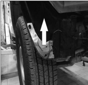
31. From right side, unstick antenna from the fender. Move antenna upper under the bar.
