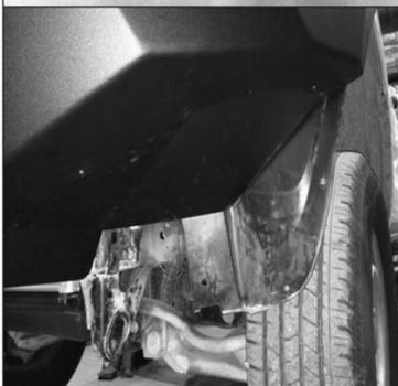
33. Install flaps using bolts M6x20 (18) and washers (24). Make sure the flaps are fixed inside of the bumper, not outside.
