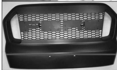
36. Cut radiator grill. First cut along the bend line. Then install the grill to the vehicle, and adjust the curve. Fix the grill after.
