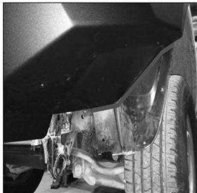
34. Push the flaps to OE plastic fenders and mark the cut line, then cut OE plastic fender.
