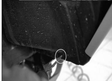
35. Mark a hole from inner side of the wheel fender from both left and right side of vehicle. Drill a 6-8 mm diameter hole.
