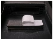
Insert radio on an angle until radio protrudes 15mm out over bottom of tray surround or insert and straighten; lay flat onto sticky back foam and apply firm pressure to top of radio with palm of hand for 30 seconds to ensure good adhesion.
