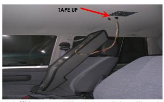
There is an 'on/off' switch located above radio opening, when 'off' it acts as a kill switch--no lights will work; when 'on' lights work independently as map/interior lights when doors are shut and timer switches off; when doors are opened, lights will work as door/interior lights.
