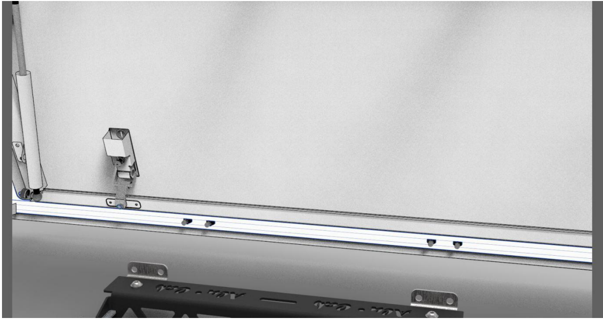
Figure 9: Hex Bolt Mounting in Canopy Nut Slot
