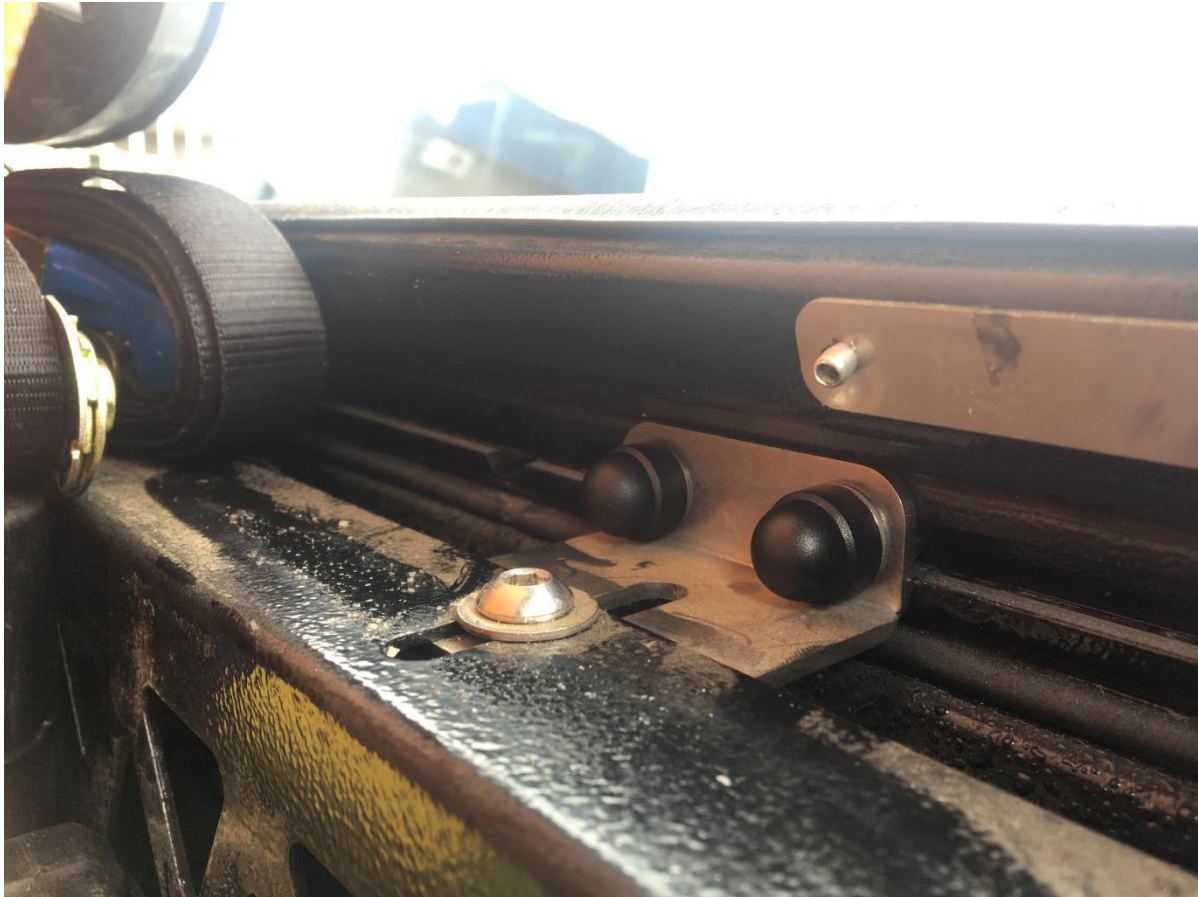
Figure 17: Side Mounting Completed with Nut Caps
