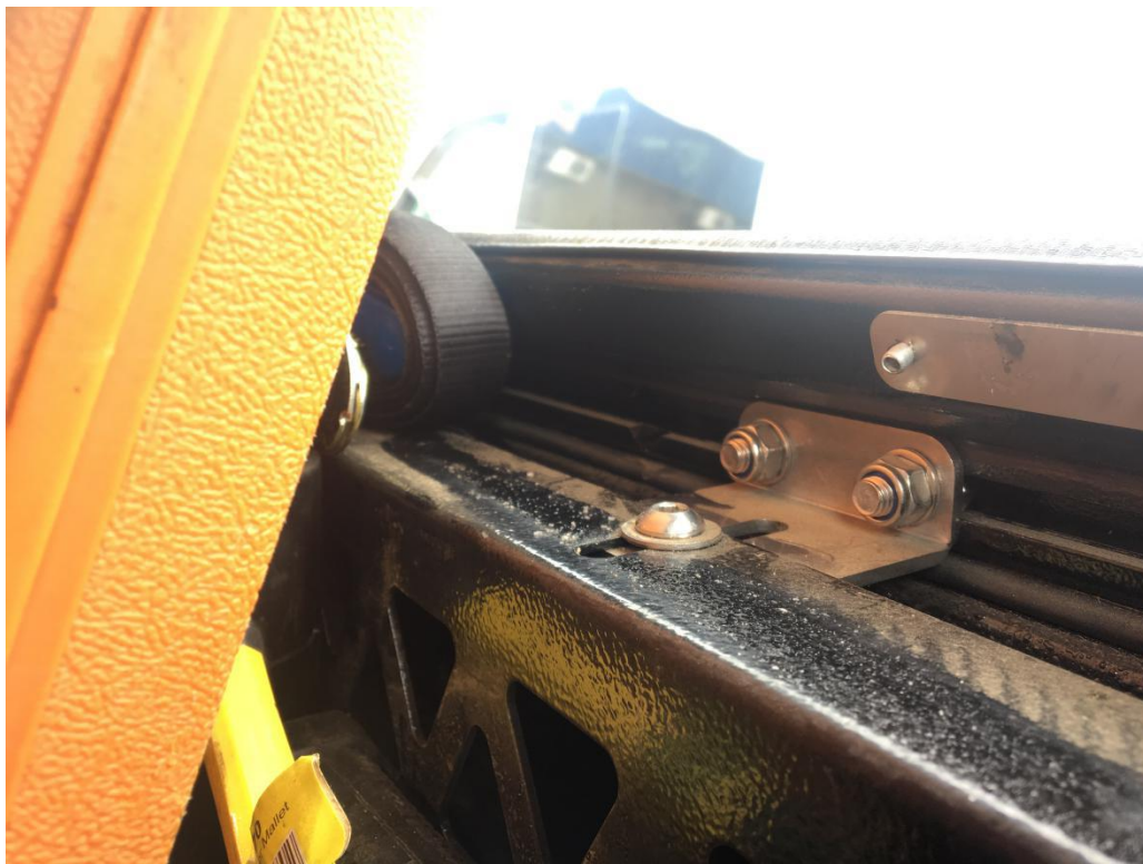
Figure 16: Chair Carrier Shelf Mounting Bracket to the Canopy Side Mounting Bracket Fastened
