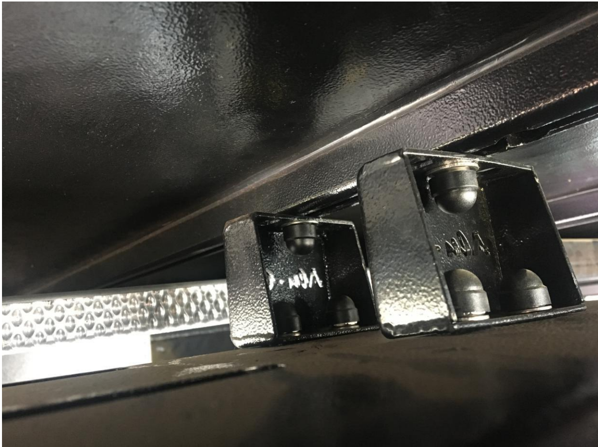
Figure 13: Place Nut Caps on the exposed Nuts
