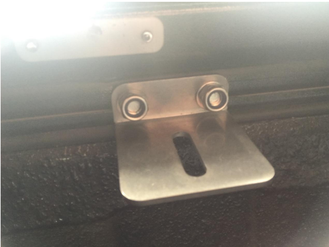
Figure 8: Finger Tighten Nyloc Nuts onto the Bolts
