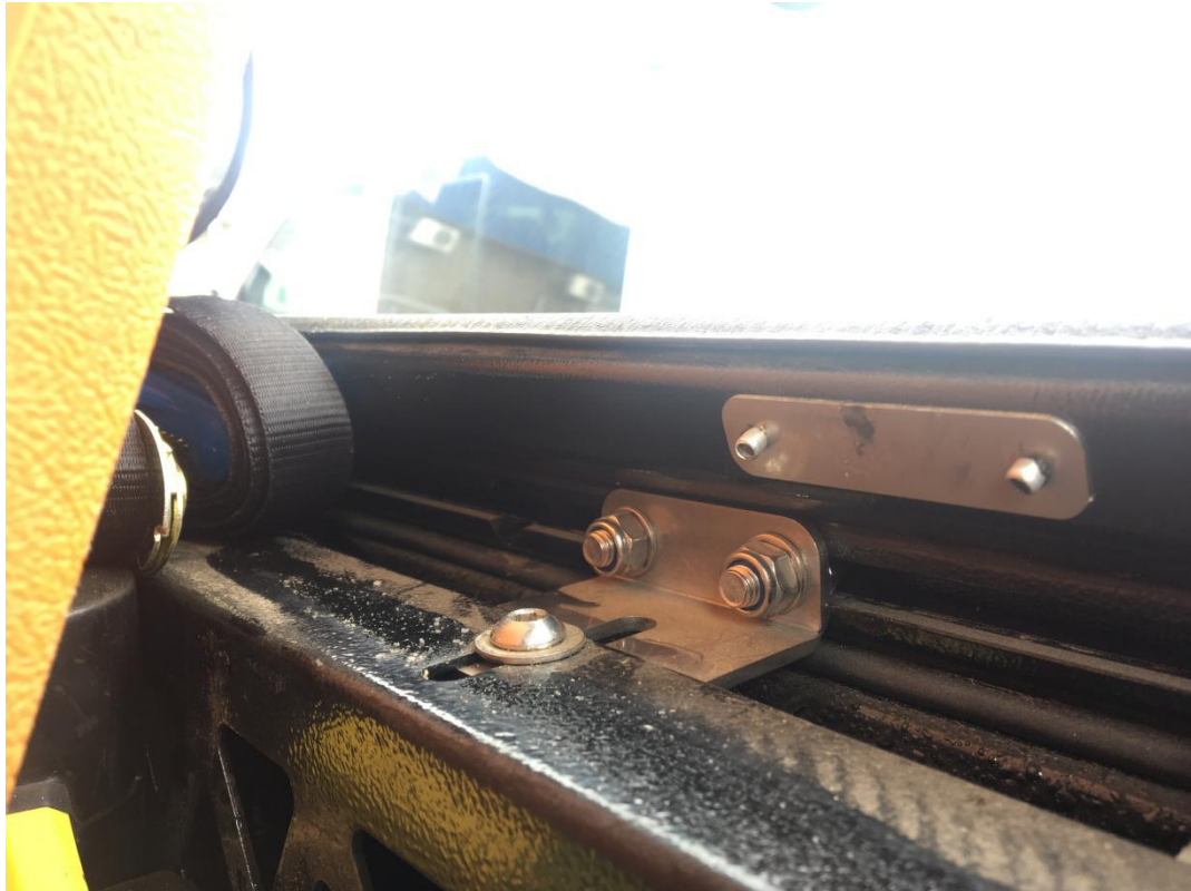
Figure 15: Button Head Cap Screw securing the Chair Carrier Shelf Mounting Bracket to the Canopy Side Mounting Bracket
