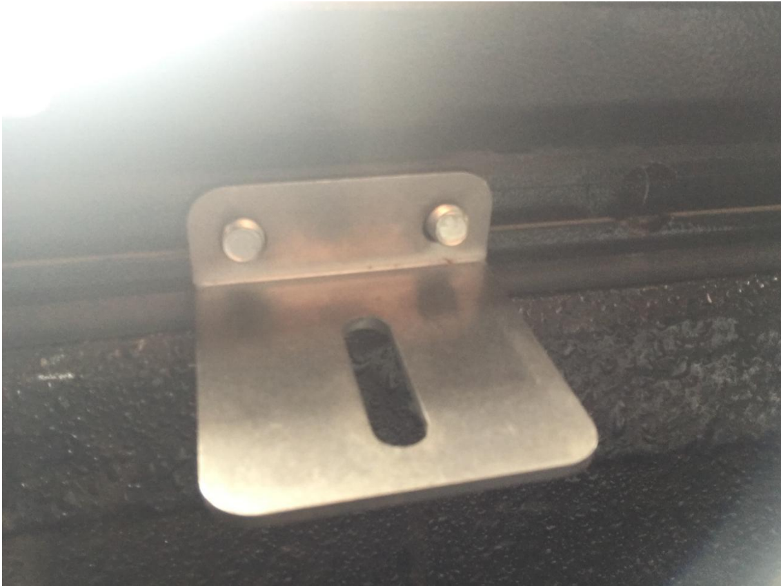
Figure 5: Hex Bolts inserted into Canopy Side Nut Slot and Bracket Positioned
