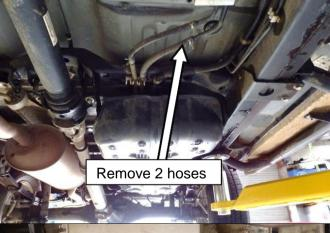
Disconnect 2 fuel hoses from the steel fuel lines, (supply and return) at front of original tank.
