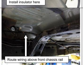
Relocate the fuel sender wiring so that it is positioned above the front fuel tank mounting on the chassis rail.
