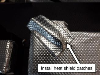
Remove the adhesive cover from the 2 heat shield patches supplied in the kit. Install these patches over the 2 brass fittings moulding them in place.
