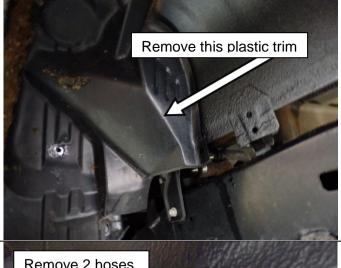
Remove plastic trim from inside LHR wheel arch to expose steel fuel filler neck.
