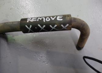
Remove the protective sleeve from the 16mm breather hose.
