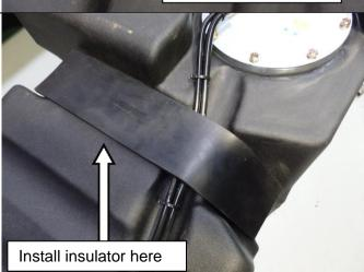
Remove the white cover from the adhesive on the 300mm long insulator pad and install this pad over the fuel lines as shown.
