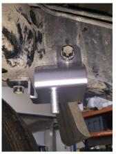
Remove the original rear strap mount adaptor from the chassis by removing the 2 M12 bolts. Secure the new mount adaptor using the same bolts.
