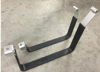
Install 2 pieces of tanks strap insulating rubber to the straps as shown.
