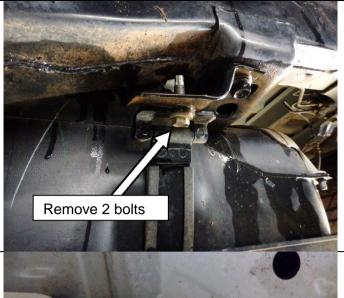
Remove 2 x M10 bolts securing the tank mounting straps to the vehicle.
