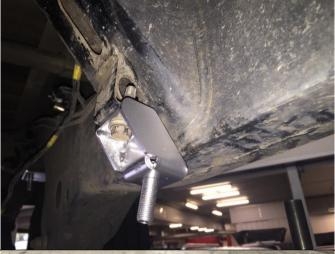
Using the original strap mounting bolt, mount the front strap mount adaptor to the chassis rail as shown.
