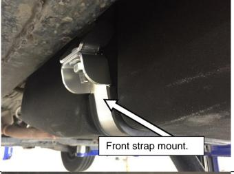
Swing front strap under tank and secure to front strap mount adaptor using the M12 nylock nut and flat washer supplied.
