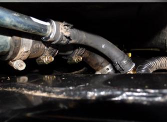
Re-install 35mm and 16mm hoses to filler neck and tank. Secure using clamps retained from tank removal procedure.
