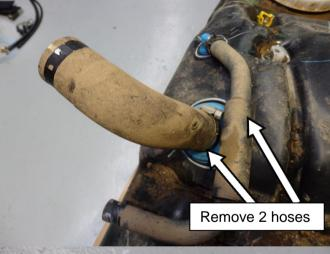
Remove 35mm fill hose and 16mm breather hose from original fuel tank.
