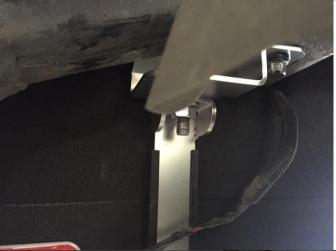
Swing the rear strap under the tank and secure the strap to the rear strap mount adaptor and secure using the M12 nylock nut and flat washer supplied.
