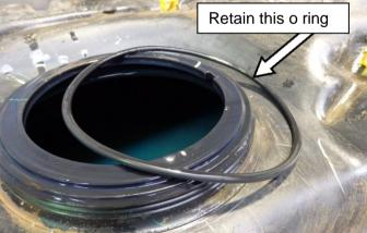
Remove the o ring gasket from the original tank and retain this o ring for the installation process
