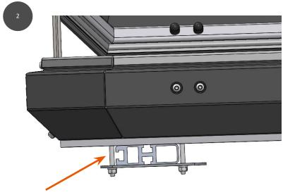
40mm long t-bolts for standard alu-cab load bars, 70mm long used for other manufacturers with a higher profile load bar.
