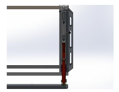
Please ensure that both brackets that are attached to the Camper, are level, as it is important for the tables moving mechanisms. Inner hole position is for DC and XC configurations and the outer holes are Land Cruiser configurations.
