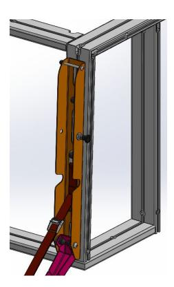
For fitment to a camper with a rear molle plate. remove the molle before positioning the side maxtrax table bolts. The center bolt will be used to bolt the molle, table bracket and cam buckle strap.
