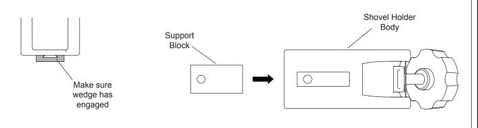
Assemble Shovel Holder to Bracket: Fit shovel holder to the bracket with the hardware provided. Be sure when tightening the bolt that the channel nut sits in the correct orientation as shown, you may need a shifting spanner to stop the channel nut from turning.
