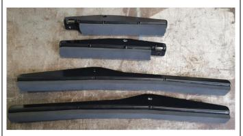
24. Fit the foam seal on the feet. Using a 7.0mm drill bit, drill through the mount feet holes to open up the foam seal.
