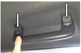
2. Remove the front and rear roof grab handles. This is done by removing plastic covers to expose the torx head screws.
