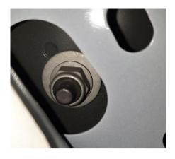
13. Remove the aluminum gutter trims from the roof. There is a large nut on the ends of each trim on the inside of the roof skin.
