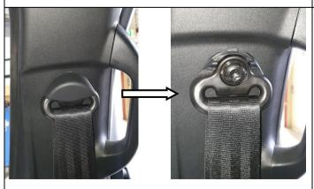
4. On the B-pillar, remove the plastic cap to expose the retaining bolt on both front seat belts.
