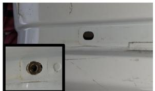
16. Using a rivnut gun, fit rivnuts to the front and rear holes on both roof gutters as shown.
