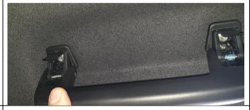
3. Remove the centre cap of the rear window hooks and rotate 45deg.
