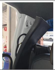
The interior roof lining needs to be dropped to install the cab rack kit.
