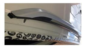
14. Remove the rear pieces on each roof gutter
