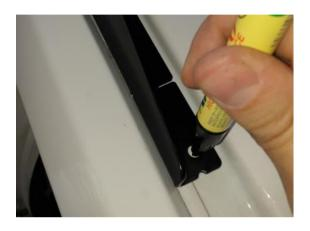
19. Use low tack film or similar to protect the areas around holes that need drilling as shown.
