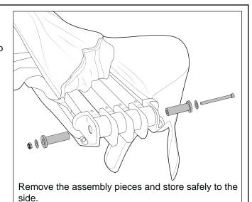
2b Using a phillips head screw driver, remove the screw holding the damages hinge moulding in place. Replace with the spare hinge provided.
