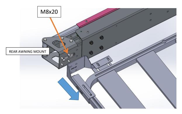
Line up the supplied brackets and and the awning to check that the awning's 270deg arm clears the vehicle.
