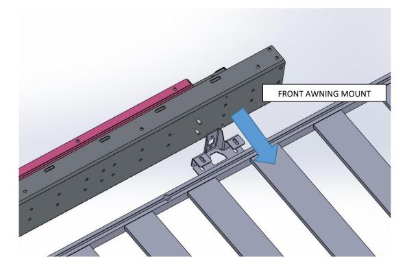
Test fit the front bracket supplied and mark the holes required to mount the awning.
