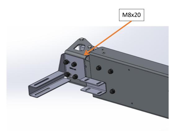
Pre-mount and fasten the rear mounting bracket to the awning with the M8 fasteners supplied.
