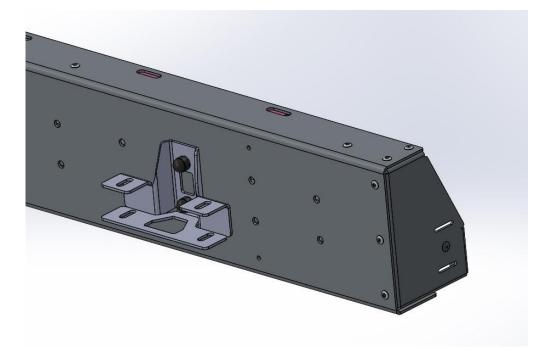
Pre-mount and fasten the front mount to the drilled holes.
