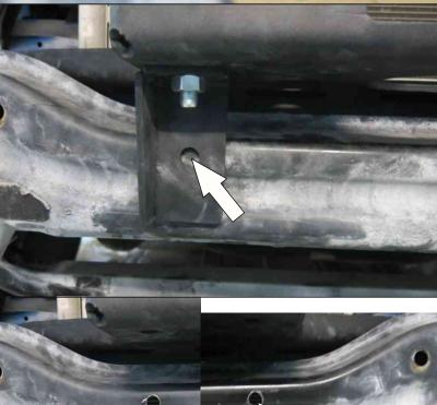
17. Mount brackets #2 and #3 to winch bracket using bolts M12x30, nuts M12 and washers #11. Mark future apertures on the front cross-bar.
