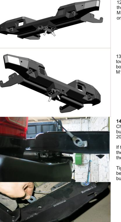
12. Instal the towing bar bracket on the car and screw with 2 bolts M12x1,25x30 and washers M12x24 on several turns.
