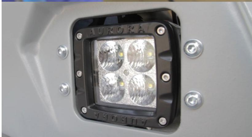
5. Install lights and brackets into the bumper facia using screws M6x16 (pos.6) and washers 6 (pos. 8). Adjust the position of lights.
