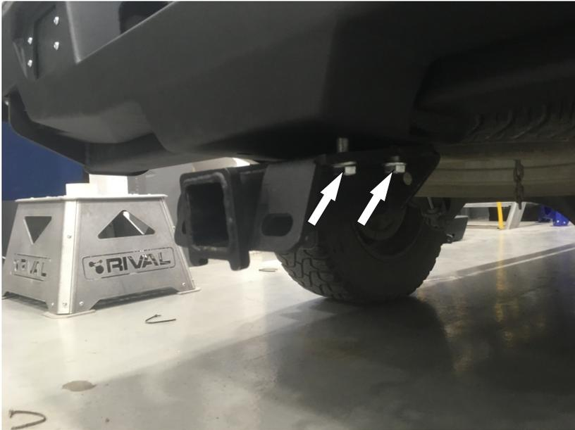
9. Install the tow bar square using bolts M12x40 (pos.11) and washers 12 (pos.12) on two sides. Tighten all screw joints.
