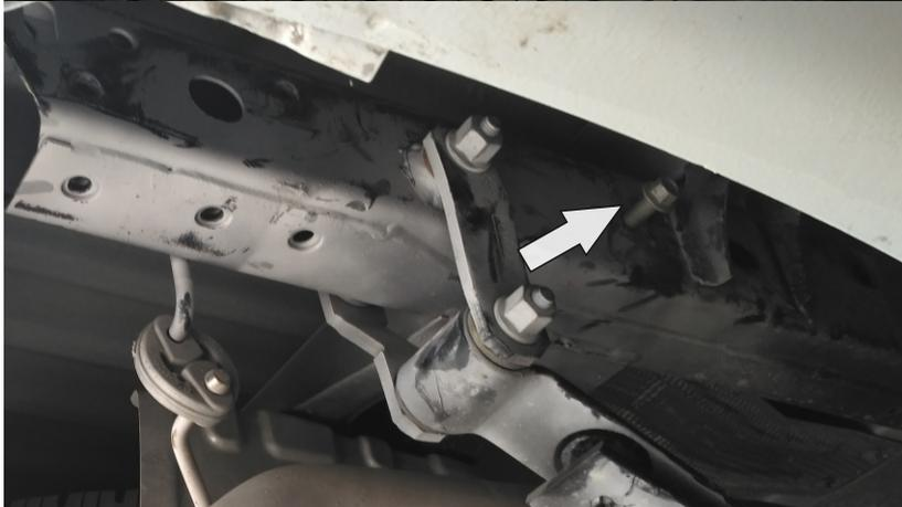
6. Install two standard tension bolts of the bumper far away from the bumper. Screw in with several revs.
