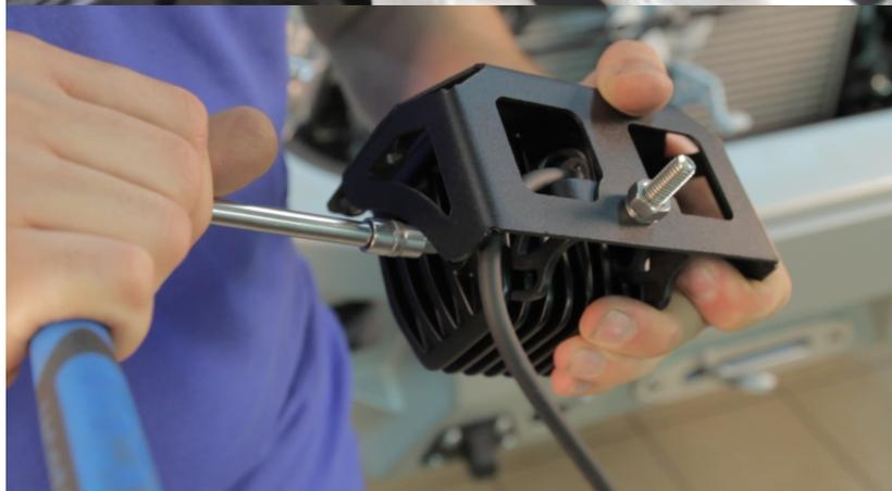
4. Install the lights (pos. 5) onto the brackets (pos.4). Align the position of lights and tighten screw joints.
