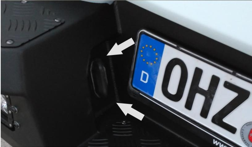
\*10. Install license lights into the fascia. Secure with screws M5x16 (pos. 15), nuts M5 (pos. 16) and washers (pos. 17).
