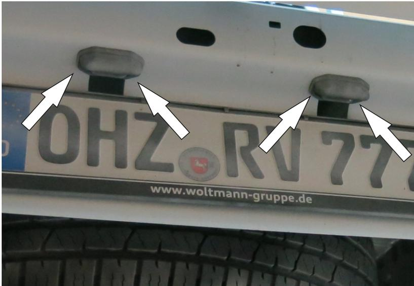
5. Unscrew self-tapping screws of the license plate lamps.
