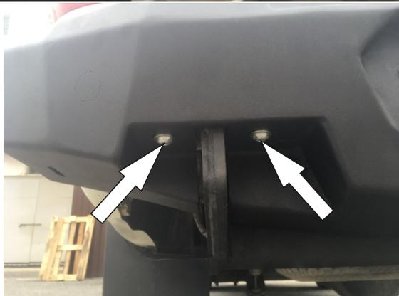
8. Install the bumper fascia (pos. 1) onto the bracket and secure it in the towing eye area using screws M10x30 (pos. 7) and washers 10 (pos. 9).
