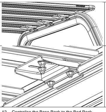
10. With the aid of an assistant, place the base rack onto the Bed Rack and align studs with the slots in the mounts.
