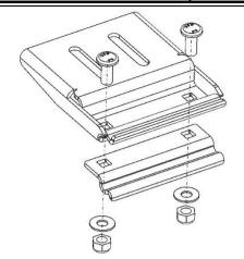
1. Install M8 coach head screws, washers and nyloc nuts through clamping brackets as shown for all six mounts.
