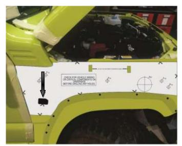
12. Cut out the outer guard template and carefully align it with the guard edges and indicator cut out (arrowed).
