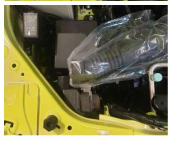
Cover the engine intake pipe with a clean plastic bag or similar so no foreign matter can enter the engine
