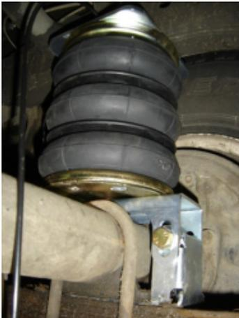
**RENFORT DE SUSPENSION PNEUMATIQUE ARRIERE (BOUDINS) POUR MAN TGE OU VOLKSWAGEN CRAFTER PROPULSION ROUES JUMEELES 4X4 A PARTIR DE 2017 (SANS COMPRESSEUR)**
