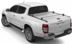
**BARRES DE PORTAGE POUR COUVRE BENNE
