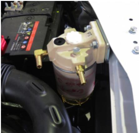
**KIT DE MONTAGE N4 POUR PRE-FILTRE RACOR POUR DACIA DUSTER 1,5 DCI A PARTIR DE 2018**
