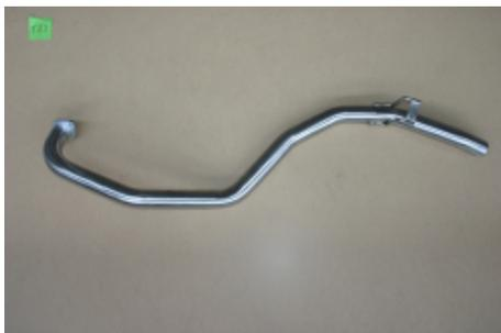
**ECHAPPEMENT INOX : TUBE ARRIERE (MODELE
