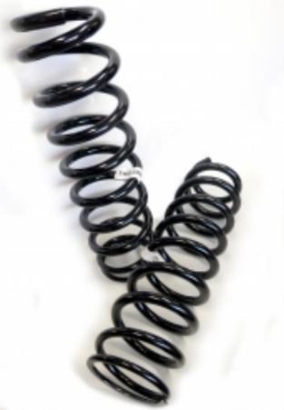
**RESSORTS HELICOIDAUX SMART COILS AVANT
