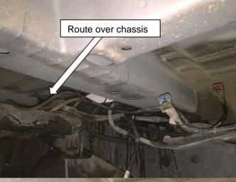
Reconnect the return line (red clips) to its original point at the rear of the fuel tank.
