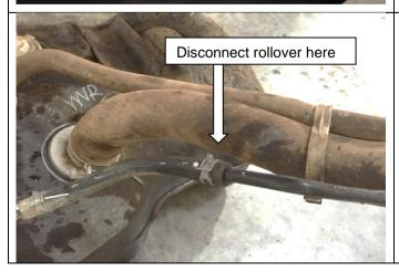
Remove the 35mm fill hose form the original tank. Retain the hose and clamp.
