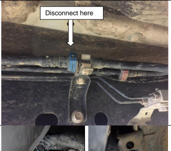
Disconnect the fuel supply line (blue clip) at the point shown in front of the fuel tank on the LH chassis rail.
