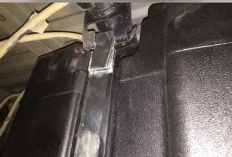
Insert the hook end of the rear mount strap into the saddle in the chassis. Swing the strap around the tank and secure using the bolts retained from the removal procedure.
