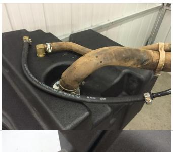
Install the 35mm and 16mm hoses onto the new tank and secure with clamps retained during removal.
