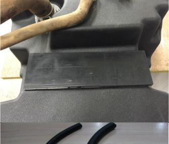
Remove the white adhesive protector from one of the rubber insulating pads and install in the position shown near the rear of the tank.
