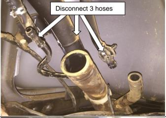
Disconnect 35mm fill hose, 16mm breather hose and 6mm rollover hose.
