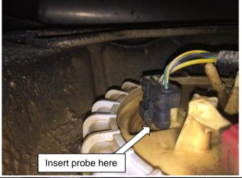
Whilst lowering fuel tank disconnect the fuel pump and sender wiring.
