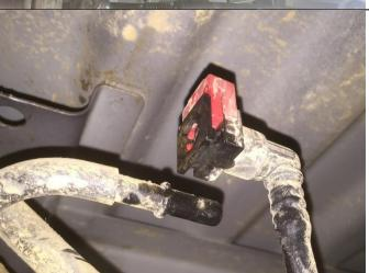
Disconnect the fuel return line on the chassis at the rear of the fuel tank.
