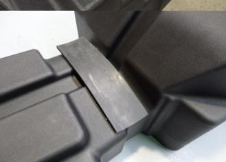
Remove the white adhesive protector from one of the rubber insulating pads and install in the position shown near the front of the tank.
