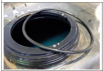
Remove the fuel pump and sender assembly from the tank and retain for the installation process.
