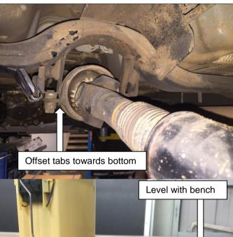
At this stage ensure correct orientation of the tailshaft centre bearing. The mounting tabs are offset and are to be positioned as shown.
