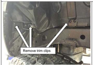
Remove wheel arch trim to expose fuel fill hoses in LHR wheel arch.
