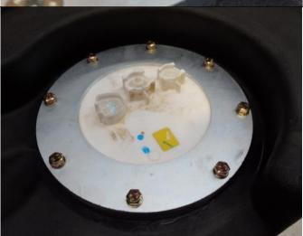
Once keyway is aligned, push the sender down into the mounting flange.
