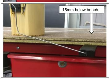
Bend the float arm down so that the top edge of the float is approximately 15mm below the top edge of the bench.
