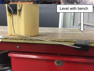
When installing a long range fuel tank to the Ranger / BT50 it is necessary to modify the fuel sender so that the vehicles Body Control Module will work with the new fuel loads.
