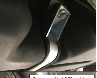
Insert the hook end of the front mount strap into the saddle in the chassis. Swing the strap around the tank and secure using the bolts retained from the removal procedure.
