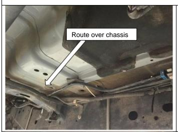
Reconnect the front end of the fuel supply line (blue clips) to the original point on the LH chassis in front of the tank.
