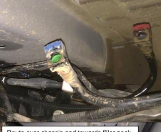
The 2 fuel pump ends of the supply and return lines should now be positioned next to each other.
