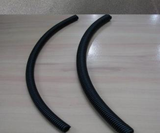
Install the 2 pieces of split tubing supplied in the kit over the top of the original fuel lines prior to reinstalling fuel lines into vehicle.
