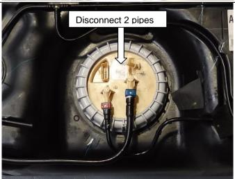
With the tank out of the vehicle, disconnect the fuel supply and return pipes and remove them from the original tank.
