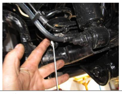
Remove brake and ABS sensor line bracket from axle housing.
