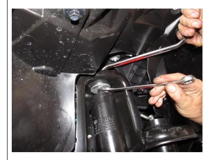
Undo shock absorber top mounting bolt.
