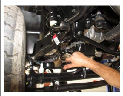
Raise vehicle until springs are no longer captive. Take care to ensure that brake lines and ABS wires are not over stretched.
