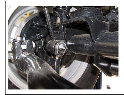
Remove the front sway bar links on both sides of the vehicle.
