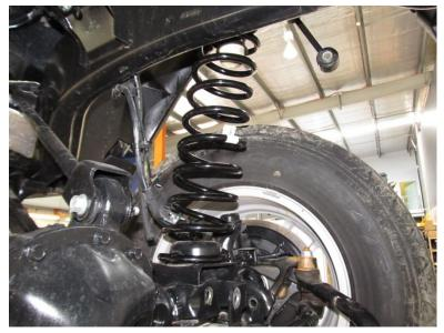
Carefully lower vehicle to compress suspension.
