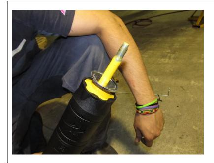
Fit retaining washer and one bushing to the top shock absorber stud.
