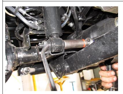
Undo shock absorber bottom mounting bolt.
