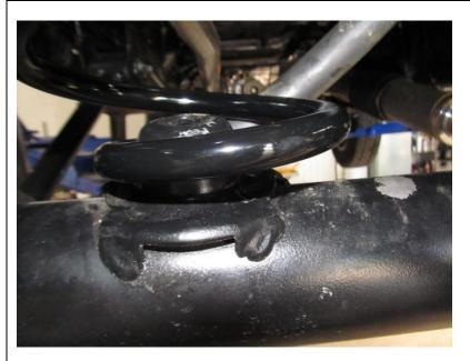
Align spring assembly on bottom seat.
