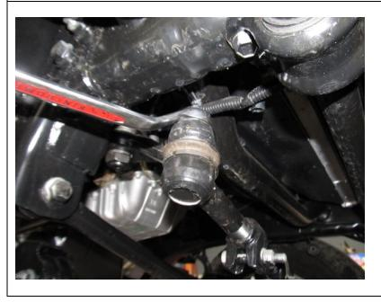
Disconnect steering drag link from the pitman arm. Hold ball joint from spinning with Allen key end of threaded section.
