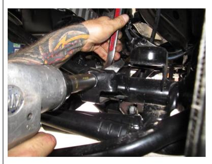
Remove bolt that connects front panhard rod to the axle housing.
