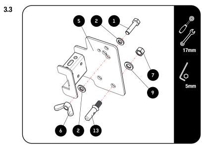
Assemble the machined pin and securing bolt in hole patern suited to your jack.
