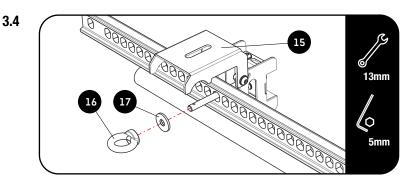
Fit and Secure the handle clamp in the desired position, using fasteners shown in Figure 1.2
