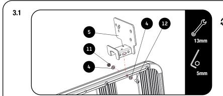
Fit and Secure Base Bracket in desired position as shown.
