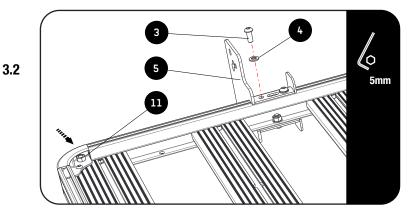
Secure as shown. Insert 2 M8 Hex Nuts at the point indicated by the arrow.
