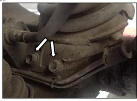
**Step 6.** Fasten all hardware including the one that secures brake line support bracket. For vehicle with electronic diff locker fitted to it, reuse original hardware. Otherwise use the picture below as guide.
