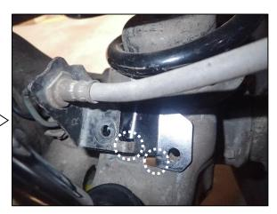
**Step 5.** For vehicles with an electronic diff lock, remove hardware shown in the picture then follow the previous step. Fit the diff lock wire bracket on the top of the new bracket.
