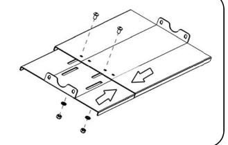
( **B** ) Open the Draw and place the Divider Plates into the Draw with the Slotted Plate to the rear. Line the Divider Plates up with Hole Sets 1 or 2 as indicated. Slide the Divider Plates apart, up against the sides of the Draw.
