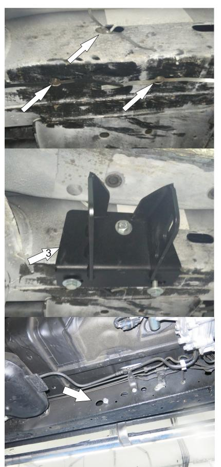
1. Place insert nuts with wires in front part of the chassis near the cross-bar.
