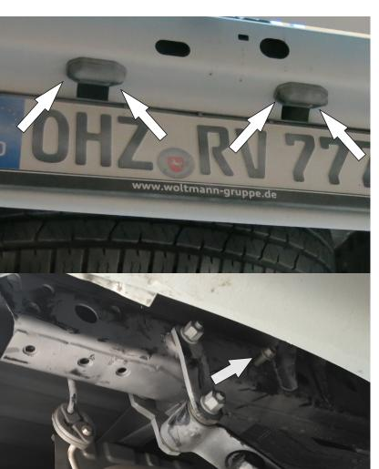
5. Unscrew self-tapping screws of the license plate lamps.
