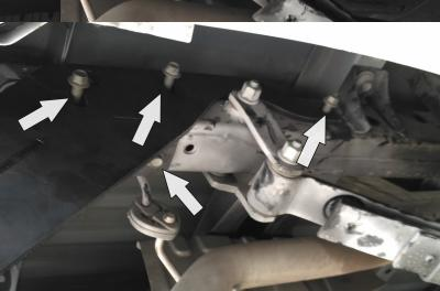
7. Install the bracket onto completed bolts. Secure it using standard tension bolts of the bumper.
