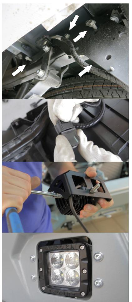
1. Unscrew tension bolts of the standard under-run bar the left and right of the vehicle frame. Dismantle the bumper.
