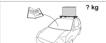
When these roof racks are to be used on a vehicle that is driven off sealed roads the maximum load rating must be divided by 1.5. Remember to subtract the weight of the roof racks to determine your maximum permissible load capacity.
