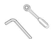
Using the M6 Capscrew, M6 Spring and Flat Washers, fix Metal RLCP Legs to the Back Bone. With the allen key provided tighten legs in place to 3-4Nm.
