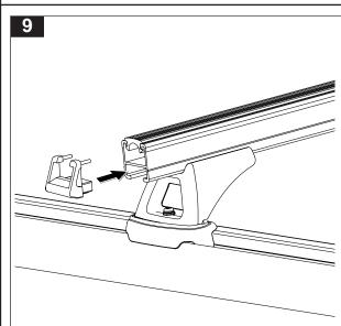
Trim the rubber buffer strip before knocking the end caps into each cross bar.
