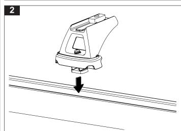
Make sure the channel nut is below the location tangs on the Jeep base pad so it can be rotated to fit between the gap in the roof rail. Sit the cross bar and leg assemblies on each roof rail.
