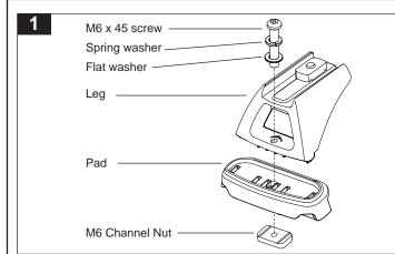
Assemble the M6 screw with washers and legs/pads as shown. Start the M6 screw with the channel nut. Leave loose. Assemble the four legs but do not tighten at this stage.
