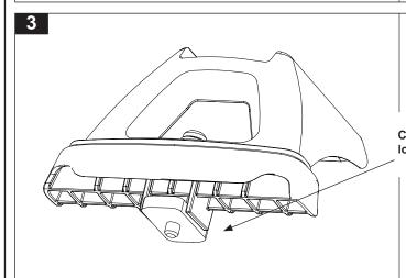
Use the security allen key to carefully rotate the channel nut until it locates between the long tangs that extend from the bottom of the Jeep base pad.
