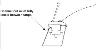
Before tightening, slide the legs to an appropriate position. As a guide use a spacing of 750-800mm.
