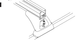
Using the security allen key provided tighten support leg attachment screws to secure the crossbars. Recommended tightening torque 3-4 Nm. DO NOT OVER TIGHTEN.
