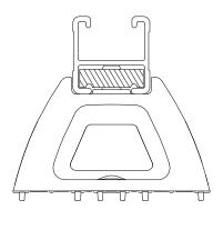
Each mounting pad is identified with a part number, position code and direction arrow. The arrow must point to the front of the vehicle.
