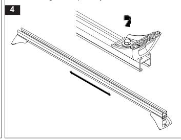
Check that the channel nut is fully located across the bar.
