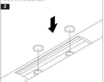
Insert the heavy duty leg assembly into the underside channel of the crossbar.
