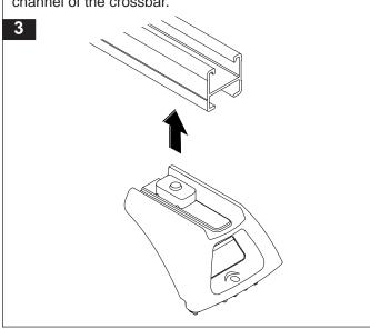
Tighten the leg attachment bolt so that the channel nut turns to locate across the crossbar. Finger tighten the bolt, as the legs will require adjustment later.
