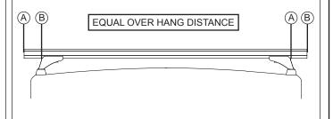
Tighten the crossbar attachment bolts. Recommended tightening torque 12-15 Nm. DO NOT OVER TIGHTEN. Check that the channel nut is located across the cross-
