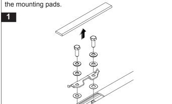
Place the 10mm large o-rings onto the plastic bolt locators in the vehicles roof.
