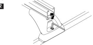
Check the crossbar over hang (A) (B) is equal on both sides, re-adjust if required. Tighten the crossbar attachment bolts. Recommended tightening torque 12-15 Nm.
