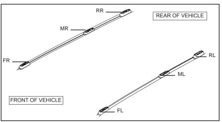
Place the M8 spring washer, M8 flat washer and 7mm small o-ring onto M8 screws. Ensure that the o-ring is fully pushed up against the flat washer. The front and rear mounting pads use M8 x 50mm screws, the middlemounting pad use M8 x 40mm screws.
