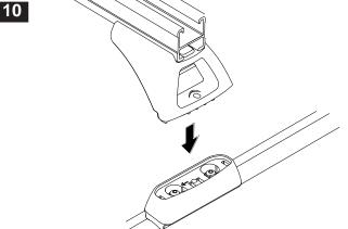
Place the M6 spring washer and M6 flat washer onto the M6 x 32mm security screw. Insert the M6 screw assembly through the support leg and screw into the mounting pad.
