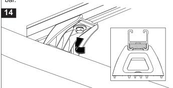
Insert the crossbar rubber buffer strip into the top of the crossbar. Insert the end caps into the ends of the crossbar, a rubber mallet may be required to fit the end caps.
