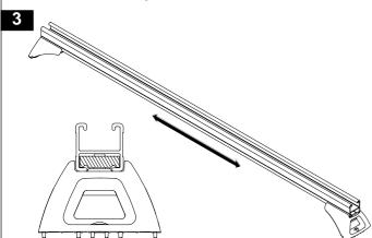
Each mounting pad is identified with a part number, position code and direction arrow. The arrow must point to the front of the vehicle.
