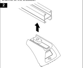
Tighten the leg attachment bolt so that the channel nut turns to locate across the crossbar. Finger tighten the bolt as the legs will require adjustment later. Check that the channel nut is fully located across the bar.
