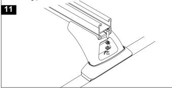
Using the security allen key provided tighten support leg attachment screws to secure the crossbars. Recommended tightening torque 5N/m. **DO NOT OVER TIGHTEN.**
