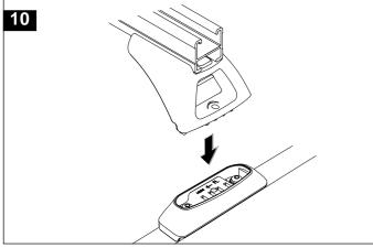
Place the M6 spring washer and M6 flat washer onto the M6 x 32mm button head security screw. Insert the M6 screw through the support leg and screw into the mounting pad.
