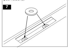
Insert the assembled screws through the mounting pads and screw into the nutserts in the vehicles roof. Tighten all screws using the allen key provided. Recommended tightening torque 6N/m. **DO NOT OVER TIGHTEN.**
