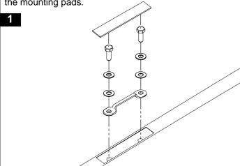
Insert the heavy duty leg assembly into the underside channel of the crossbar.
