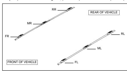
Place the M8 spring and flat washer onto the M8 screw. Place the O ring no to the screw and push the O ring up against the flat washer. The front and rear mounting pads use M8 x 50mm button head screws and the middle-mounting pads use M8 x 40mm button head screws.
