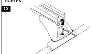
Check the crossbar over hang (A) (B) is equal on both sides, re-adjust if required.
