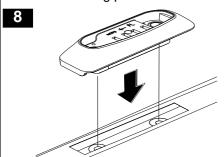
Place the mounting pad washer gasket in the gutter recess and align the hole in the washer gasket with the mounting pad nutserts.
