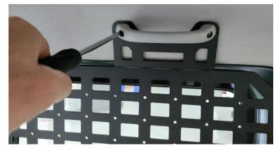
If no original handle are present, use the 2 X spring washers, washers and button-head bolts provided in the pack to secure the top part of the plate to the handle mounts in the vehicle.
