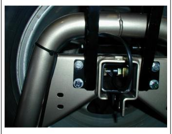
68. Cable tie loom to wheel carrier frame leaving enough excess, as shown above, for fitting to number plate bracket.
