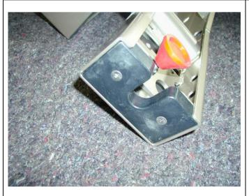
3. Fit black urethane C shaped part into end section of arm using M6 x 30 stainless steel counter sunk cap screws and nyloc nuts.
