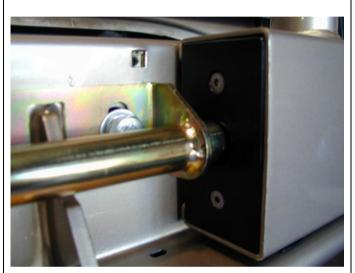
27. To adjust the position of the centre locator bracket, close wheel carrier arm so that tube sections of the locator bracket are centralised by the urethane C section.
