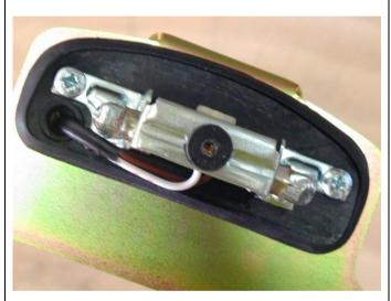
61. Secure light to bracket using M5 pan head screws and flange nuts.
