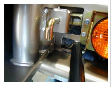
38. Using **M8 nyloc nut**, fit covered end of strut to rear bar mount and tighten securely.
