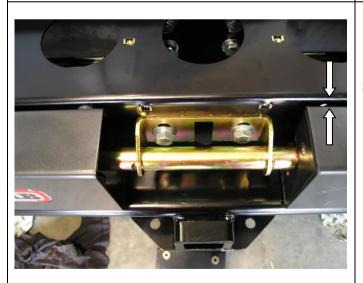
When closed and under tension the rear of the arm should be 5mm from the front face of the rear bar.
