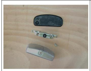
58. Remove screw from front of light and disassemble as shown.
