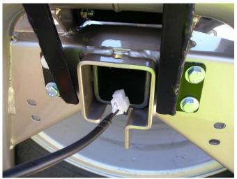
67. Feed loom through rear of wheel mount as shown.
