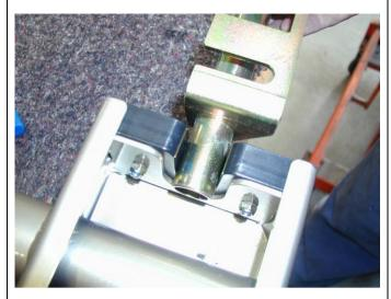
4. After tightening cap screws to secure black urethane to arm, check clearance using centre locator assembly as per photo.
