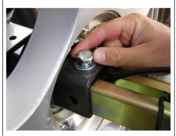
70. Secure finger tight with **M12 x 30 bolt**, spring washer and flat washer.
