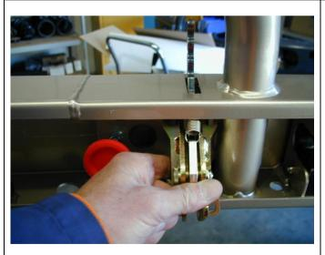
29. To fit catch assembly to arm mounting plate, pass handle through slot in top of arm and secure using four M8 x 20 stainless steel cap screws and spring washers.
