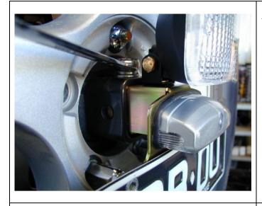
71. Slide bracket in and secure tightly.
