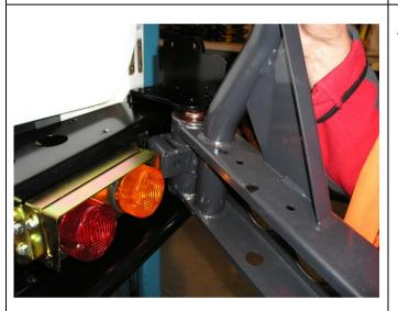
18. Slide wheel carrier arm between outer mount plates of rear bar and align holes.
