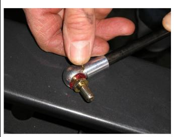
37. Fit ball mounts to both ends of strut and lock using wire retainer clips.
