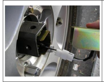
69. Connect loom and insert number plate bracket into wheel mount.
