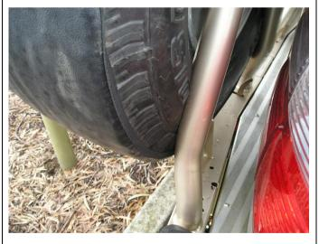
52. Push tyre so that tyre touches frame. Note the position of the wheel mount bracket in the wheel carrier.
