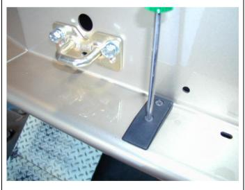
12. Tighten until head of screw is just below surface of black plastic wedge.
