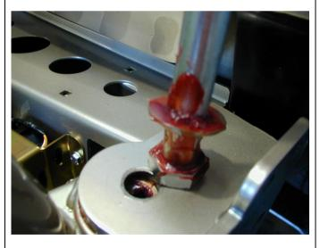
19. Fit large flat washer to M20 x 190 bolt and cover with grease as shown.
