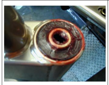
17. Cover top and bottom of bearing hub with grease to waterproof product.
