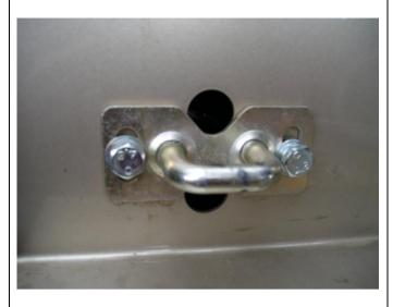
M8 caged nuts should be already fitted to rear bar. Caged nuts must be fitted to rear bar before rear bar is fitted to vehicle.
