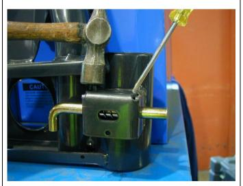
6. With the help of a friend, place a flat blade screw driver into slot on top of bracket. Force spring rearward, then holding roll pin with pointed nose pliers, fit roll pin into hole in locking pin and tap into place with a hammer until roll pin protrudes approximately 3mm through slot in top of bracket.
