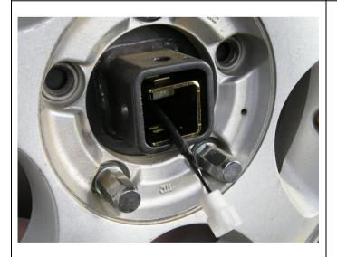
Fit M12 x 1.75 caged nut to channel then sit inside wheel mount as shown.
