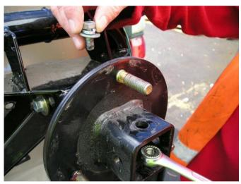
55. Once the 10mm hole has been drilled, fit a 10m x 30 mm bolt assembly ( SEMS ) into drilled hole. Fit a 10mm flange nut into a 15mm ring spanner, slide inside tube section to rear hole and tighten bolt securely.
