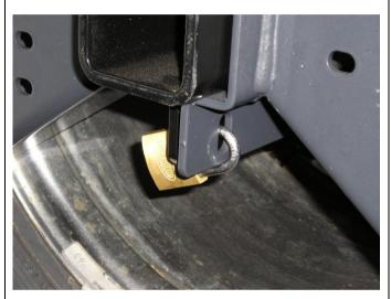
72. To secure wheel mount bracket to wheel carrier a padlock can be fitted as shown.
