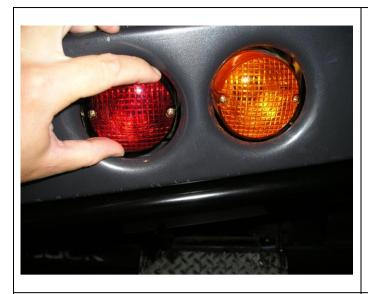
36. Centralise light assembly over apertures in arm and tighten all 6mm hardware.
