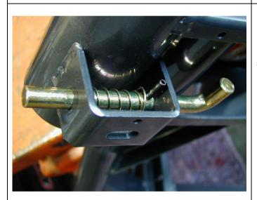
The photo shows the locking pin assembly viewed from underneath.
