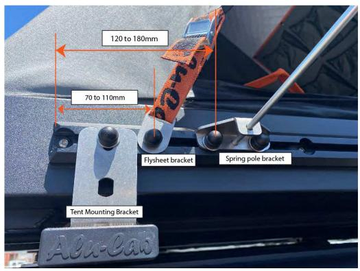
Alternatively, should you not have enough space on the leff-hand side, the Spring Pole Bracket could also be mounted on the right-hand side of the cargo rail as specified below:
