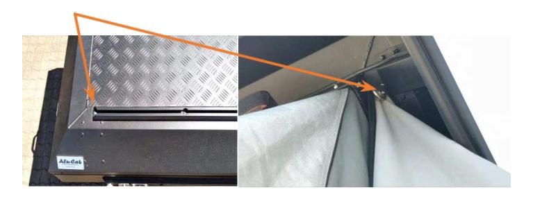
Bolt 2: (the sixth bolt from the front end of the cargo rail, situated inside the lid of the tent)
