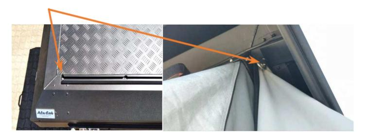
Bolt 2: (the fourth bolt from the rear end of the cargo rail, situated inside the lid of the tent)
