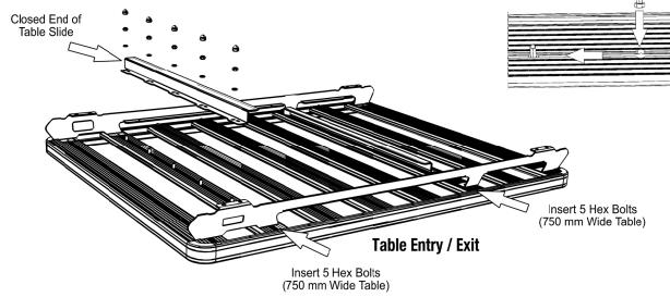
( **C** ) Space the Table Slides 250 mm in from the edge of the Rack as shown.
