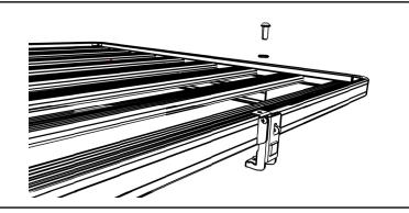
( F ) Once the Rack has been mounted to the vehicle, open the Latch by pushing on the Latch Release and slide the Table into position. A small padlock can be used through the hole in the Latch Release should you wish to lock the table.
