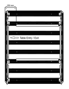
( D ) The Table Slides are slotted left to right to enable adjustment. Space the two Table Slides 750 mm apart and tighten all the Nyloc Nuts. Place a M8 Nut Cap (Item 6) over each Nyloc Nut.
