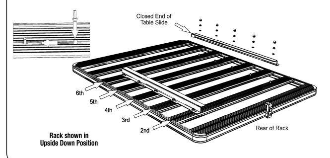
( **B** ) Space the two Table Slides 750mm apart and tighten all the Nyloc Nuts and place a M8 Nut Cap (Item 6) over each Nyloc Nut.
