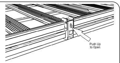
A small padlock can be used through the hole in the Latch Release should you wish to lock the table.
