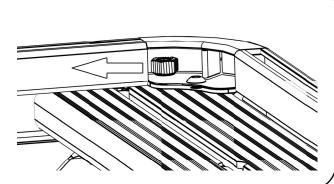
(F) Place the Latch (Item 10) onto the Rack, lining up the mounting holes in the Latch with the Nyloc Nut inserted in Step 2E. Secure the Latch in position using two M8 x 20 Button Head Bolts and two M8 Flat Washers (Items 7 & 9).
