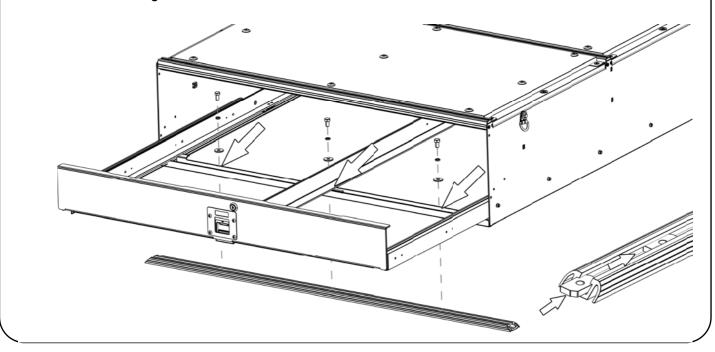
(  ${f E}$  ) Place the Drawer System into the vehicle and position as desired.
