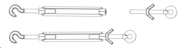
( **B** ) Assemble the M6 Eye Nuts and Nylon Washers (Items 7 & 8) to the Stud Plates (Item 9) as shown.
