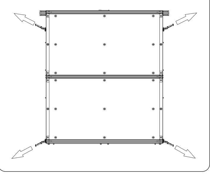
( H ) Once you have the four mounting points on your vehicle, secure the Drawer to the vehicle by tightening the four Turn buckles. Once the Drawer is secure in position tighten the Wing Nuts on the Turn Buckles and the Bolts securing the D-rings to the Drawer System and the vehicle's load bay.
