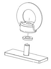
( C ) Assemble two D-rings (Item 4) to either side of the Drawer as shown using the M6 x 20 Hex Bolts, M6 x 19 Flat Washers and M6 Spring Washers as shown.
