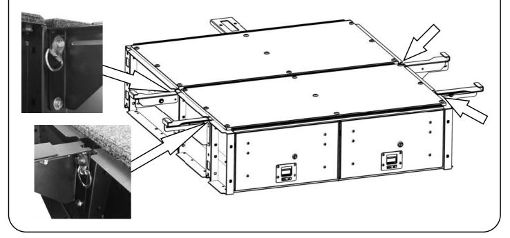
( C ) Position the Corner Wing Assemblies from Step 2B over the rear corners of the Drawer as shown. Secure the Assemblies to the Drawer using the remaining M6 x 20 Hex Bolts, M6 x 19 Flat Washers and M6 Spring Washers.
