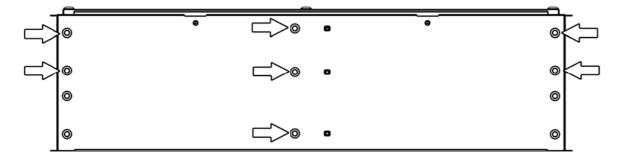
( **F** ) Using six M6 x 20 Hex Bolts, six M6 Spring Washers and six M6 x 19 Flat Washers removed in Step 2E, secure the Rear Support (Item 23) to the back of the Drawer System as shown.
