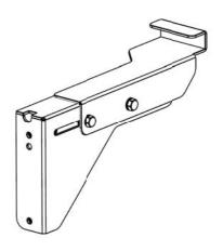
(  ${f B}$  ) Using Step 2A as a guide, loosely assemble the Corner Wings (Items 24, 25, 26) as shown.
