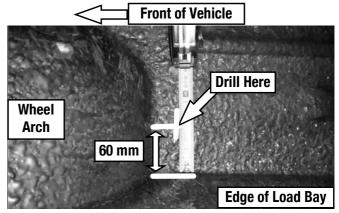
( H ) Looking underneath the left and right rear corners of the vehicle's load bay, locate the "pre - punched" hole as indicated by the arrow. Drill a 6.5 mm hole in the center of the "pre - punched " hole on either side of the load bay.
